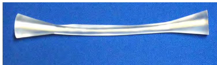
図 4-8-19 A developed test piece for radius
